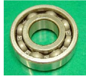
✦Bearing 伤痕检查
